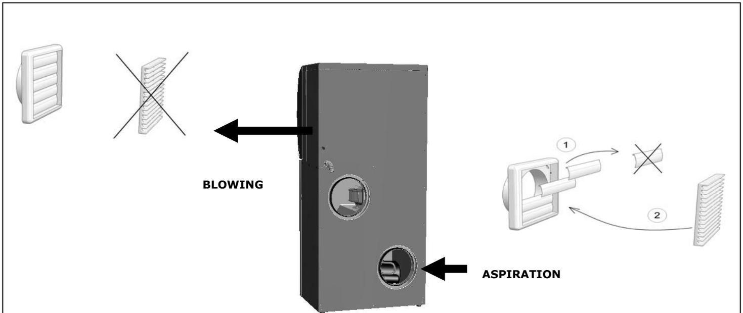
ATTENTION ! each case is composed of 2 grids (blowing and aspiration). it is necessary to adapt the type of grid
